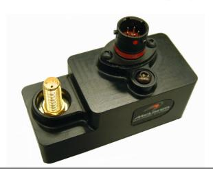
The tyre pressure receiver unit is for use with MESL tyre pressure sensors. The sensors transmit pressure, temperature, battery voltage, serial number and life count data over an RF link to an antenna on the car. Signals from the antenna are passed to the tyre pressure receiver unit where they are decoded and sent to the ECU via CAN to be further processed and scaled.
